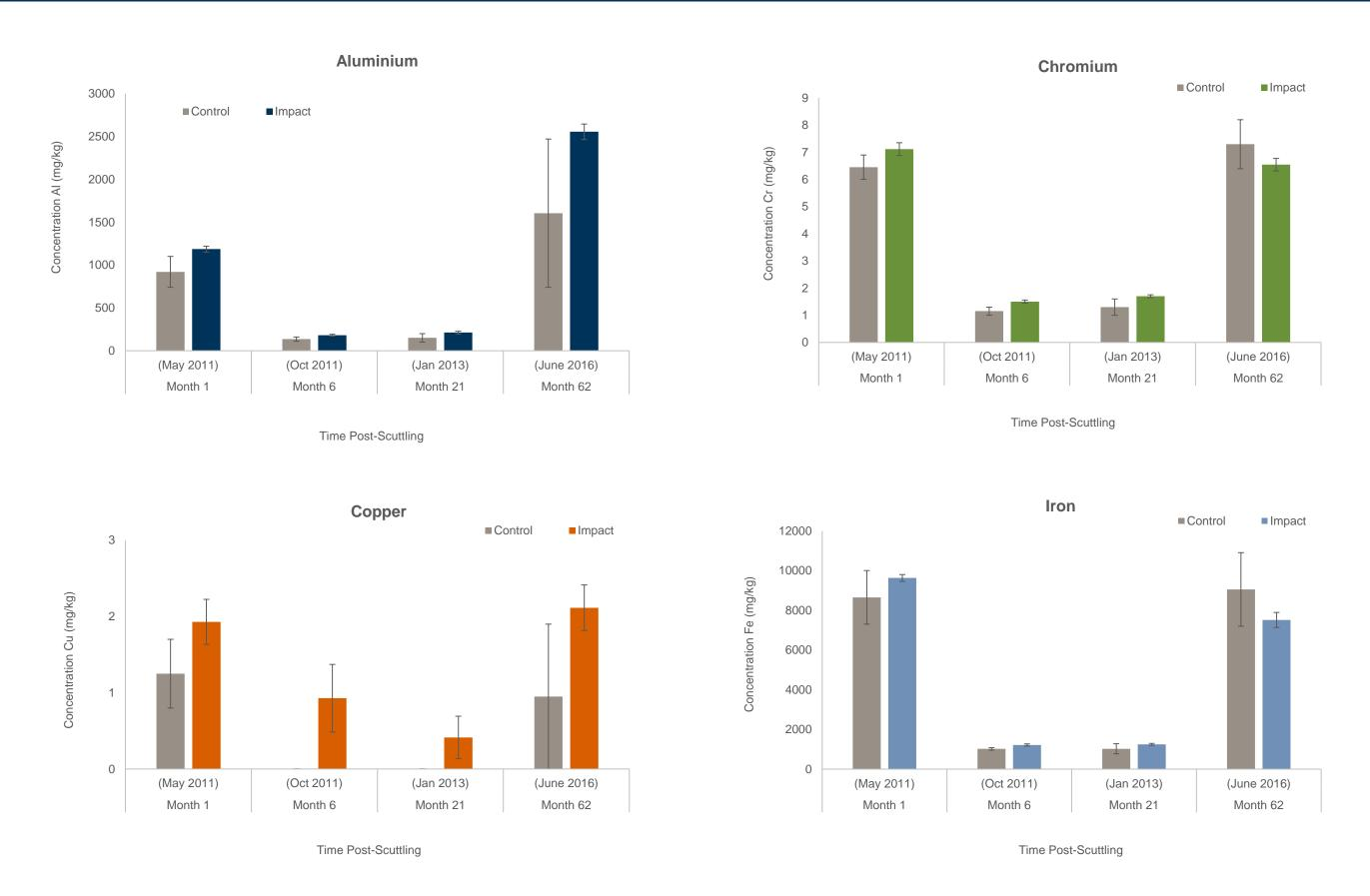
Figure 3. Mean Heavy Metal Concentrations Recorded in Sediment Samples Collected from Monitoring and Control Locations during May 2011 (one month post-scuttling), October 2011 (six months post-scuttling), January 2013 (21 months post-scuttling) and June 2016 (62 months post scuttling)
