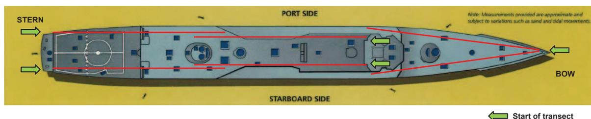
Figure 2.2 Approximate location of horizontal transects on the superstructure of the Ex-HMAS ADELAIDE (N.B. this image is diagrammatical only and is not to scale).
