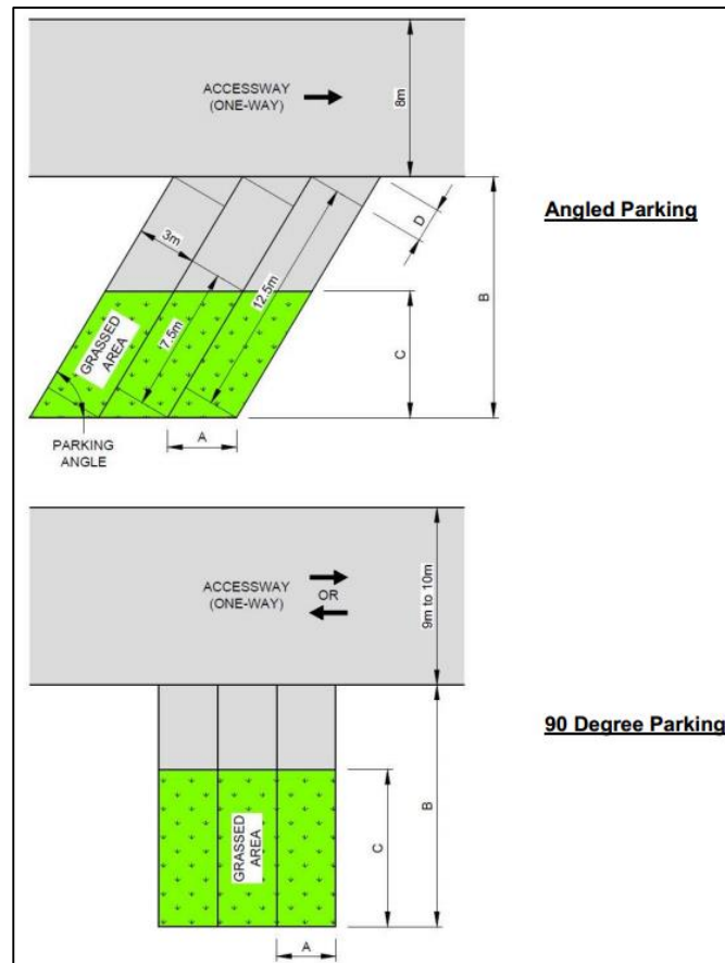
Figure 5 Typical car and trailer parking space geometry dimensions (RMS NSW Boat Ramp Facility Guidelines)
