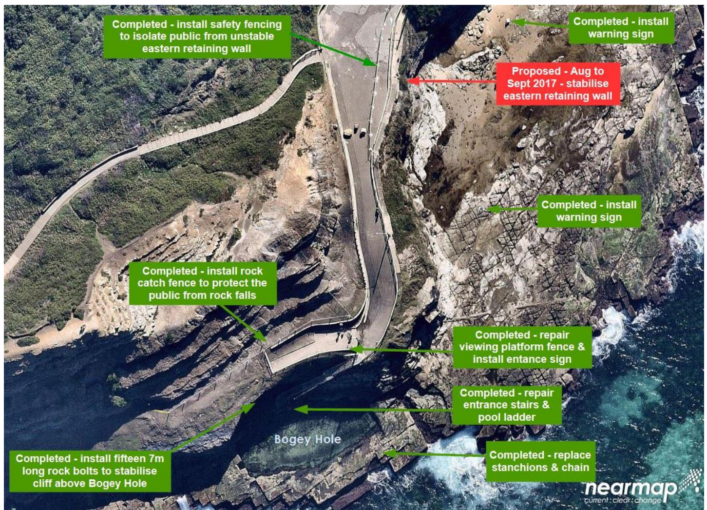
Figure 1. Plan showing Stage 1 & Stage 2 stabilisation works - Bogey Hole
