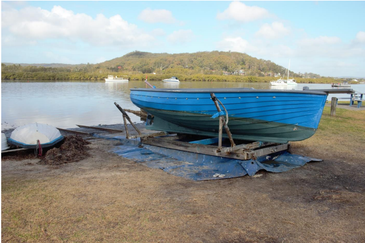
Figure 3.7 – Slipway and cradle for Putt Putt boats likely very similar to the early slipway at the Empire Bay boat shed.
