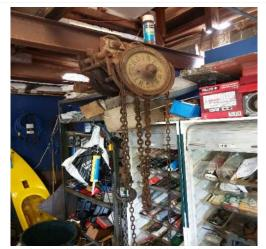
Photograph 36 shows the chain block that appears to still be in use.
