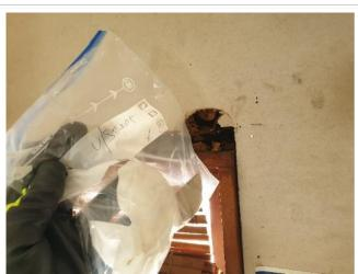
Photograph 66 shows sample taken from FC wall lining to loft / mezzanine level.
