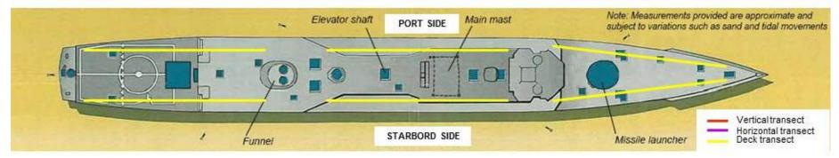
Figure 2: Plans of the Ex-HMAS Adelaide and Positions of the Reef Community Survey Sampling Transects.
