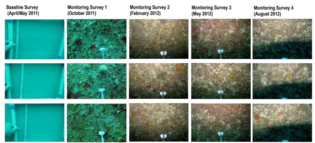
Plate 9: Vertical Hull Port Bow
