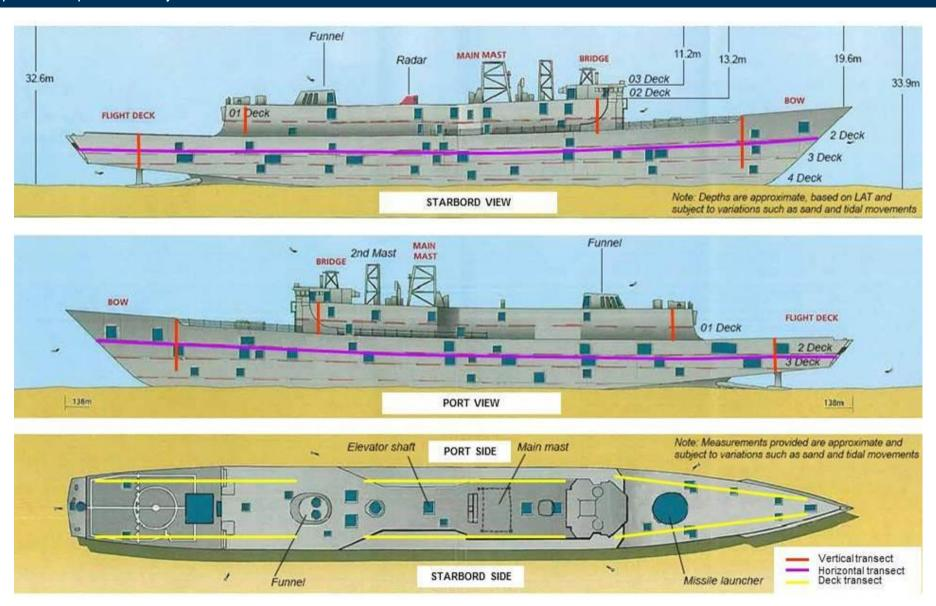
Figure 2: Plans of the Ex-HMAS Adelaide and Ppositions of the Rreef assemblage Community Survey Survey Sampling Transects transects.
